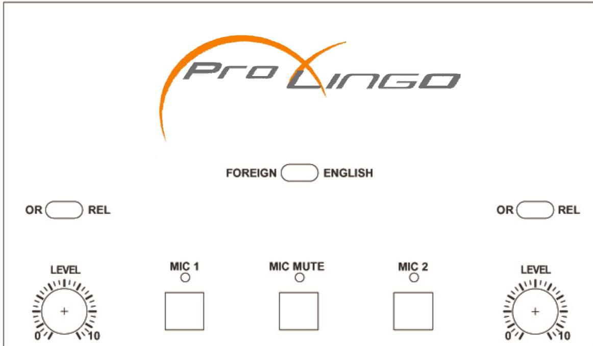
1. **FOREIGN-ENGLISH SWITCH:** Selects outgoing channel. Indicator lights indicate the selection. This switch selects between outputs OUT A and OUT B on the rear panel: OUT A corresponds to FOREIGN. OUT B corresponds to ENGLISH.
